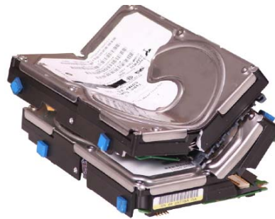
Two hard drives after destruction.
